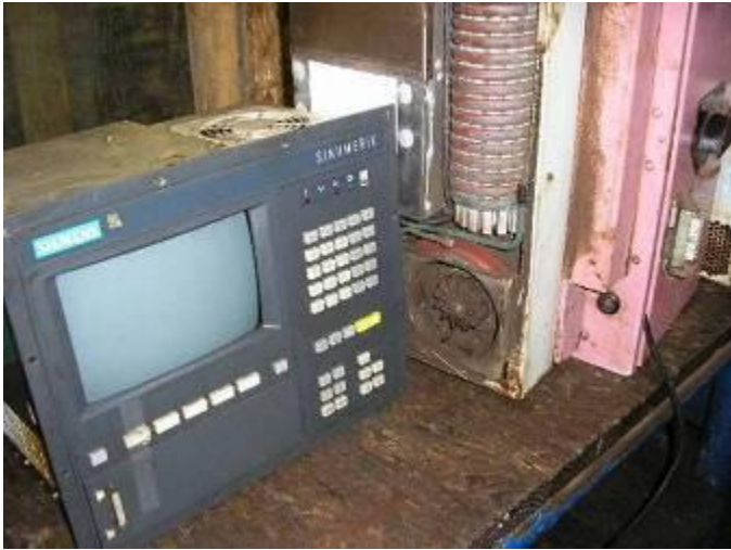
16: 20 years later no spare controller available, CNC will be replaced with a new CNC.
