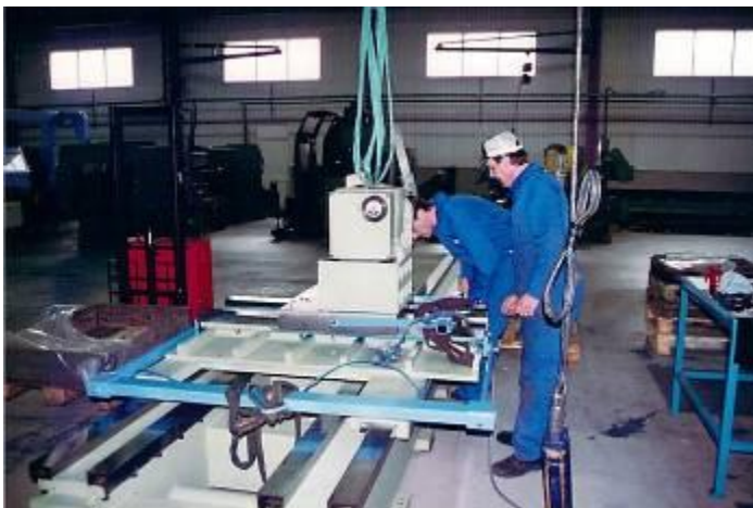
Figure 12: the carriage Einschaben X and Z axis
