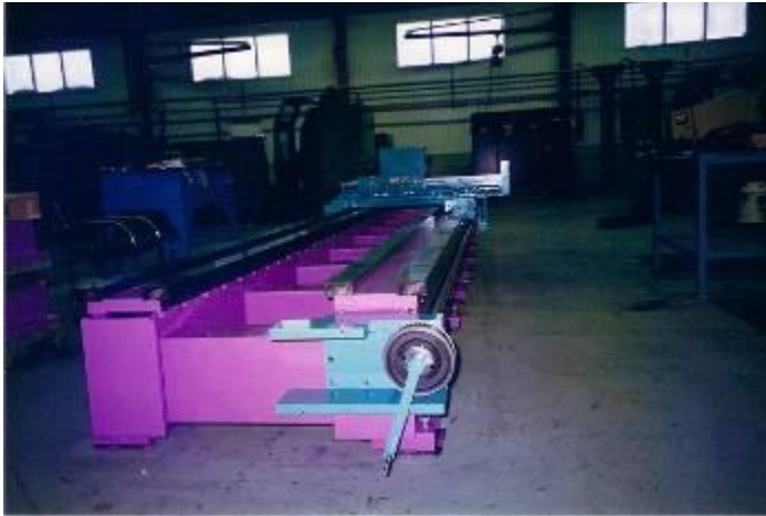
Figure 11: Construction of a new machine bed for Gornati, with cross slide.
