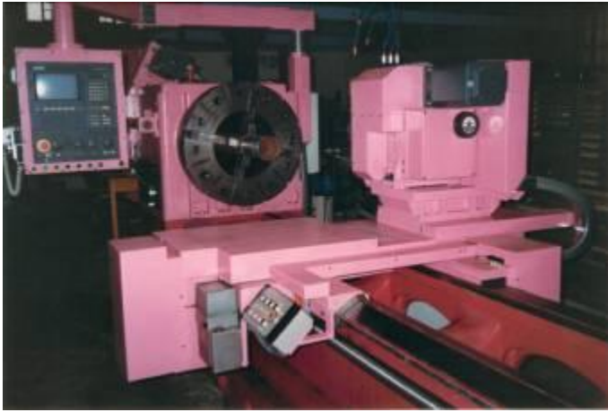
Figure 5: Construction of a new tool turret
