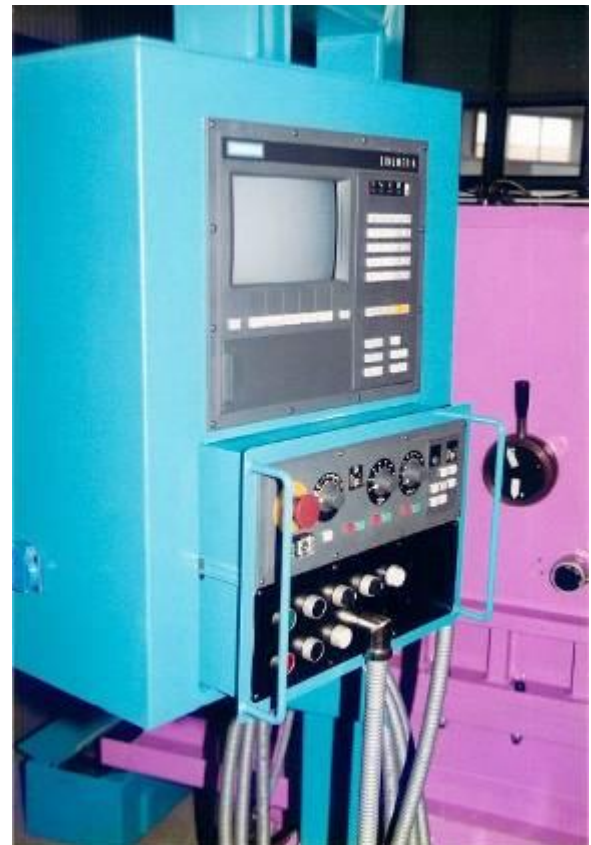
Figure 15: New CNC Sinumerik 810T with portable box.
