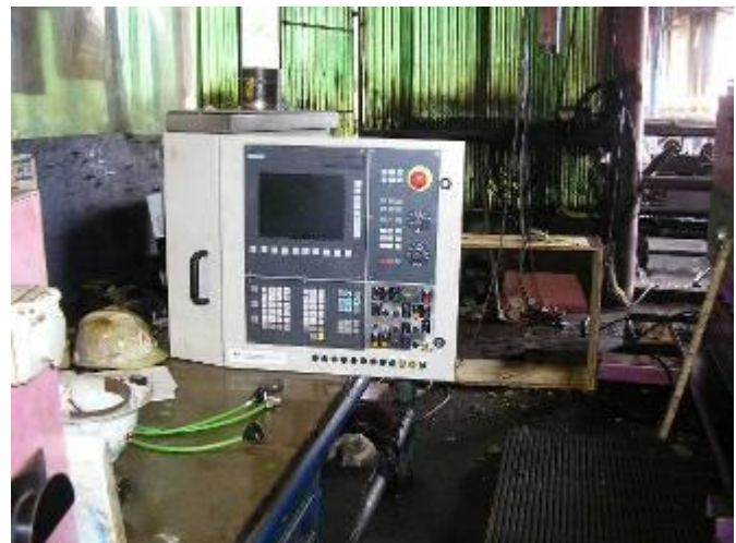
Figure 20: The new CNC control Sinuemrik 802 DSL
