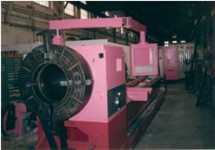
Figure 6: oilfield lathe with double lining
