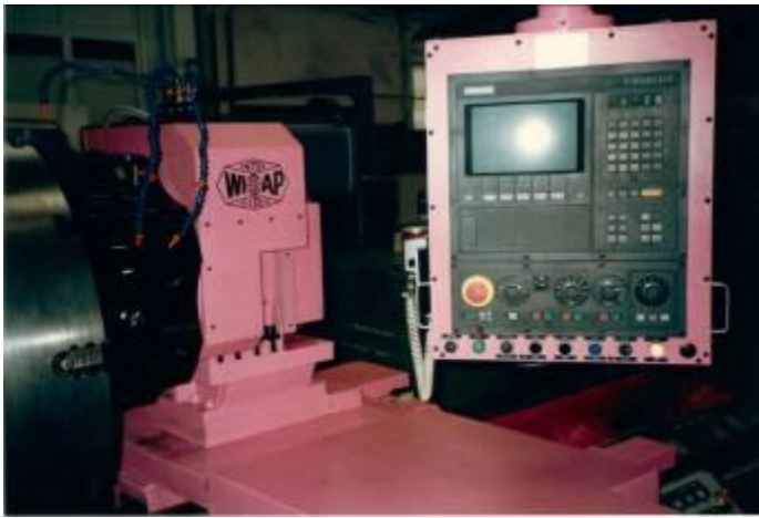
Figure 1: Total revision with retrofit. Conventional Gornati lathe system WIAP.
