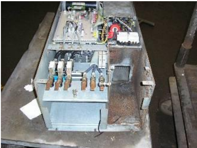
Figure 17: The Siemens feed and spindle drives are greedy from the air by the sea.
