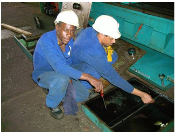
Photo: During commissioning, the lubrication will not the way we want it. No pressure build-up. Joba investigated. Then you see that the pump is faulty, so a conversion also helps error that can cause expensive consequences, are found before the damage.
