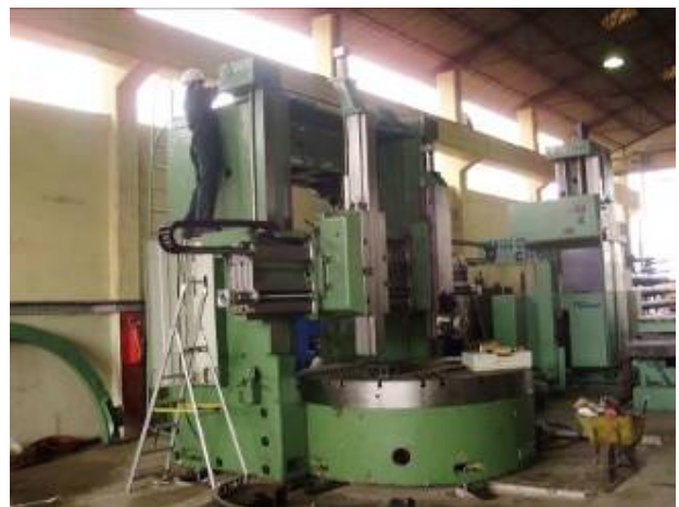
Previously a conventional vertical lathe and now new a CNC-controlled machine. WU_240_210
