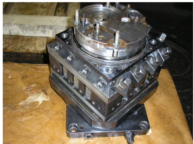
Photo: Bald ready-mounted turret, tested everything by hand, it locks beautiful. Tip top.
