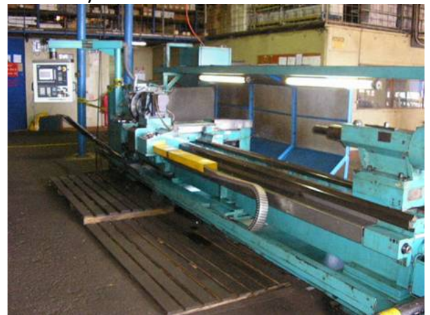
Photo: The machine in production. All were glad that with the new control could have been in production the first CNC again. What was coming with the new programs, was then aware when they saw how easy it produced over 10 years with a very simple system. All parameters programmed. A program looked it. For each oil thread like this. Enter only 15 values and a thread was ready.
