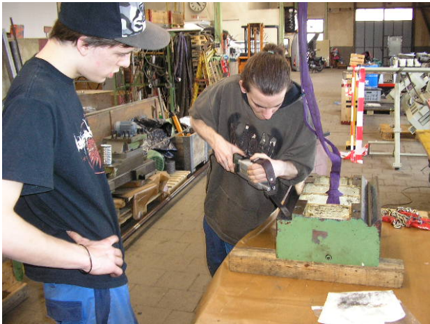
Scraping the geometry Per times about 0.004 mm
