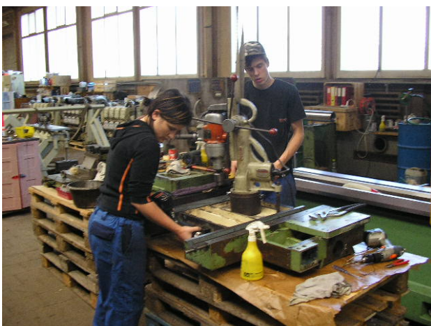
Photo: Caro drilled new lubrication holes in the sled.
