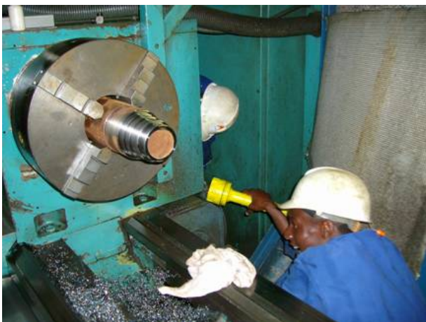
Photo: During commissioning, the lubrication will not the way we want it. No pressure build-up. Joba investigated. Then you see that the pump is faulty, so a conversion also helps error that can cause expensive consequences, are found before the damage.
