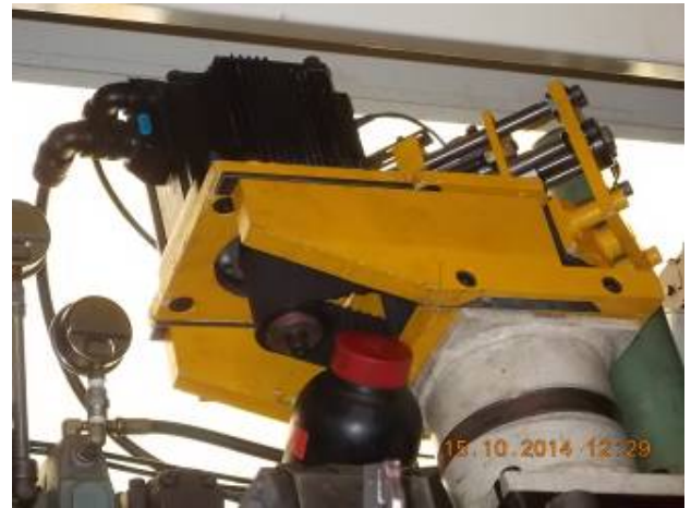
To ensure that all feed motors could be used without brakes, an external X brake was made from spare parts reasons, not in the engine.
