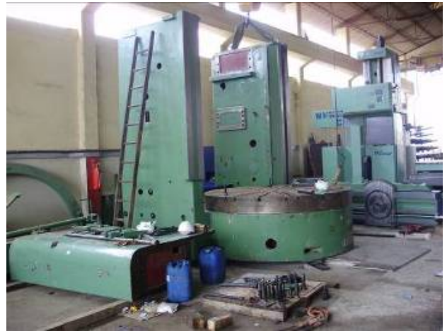
Now the second side stand is mounted. WU_240_50
